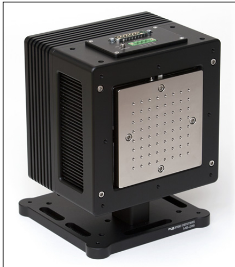
286 mounted vertically on riser and base
