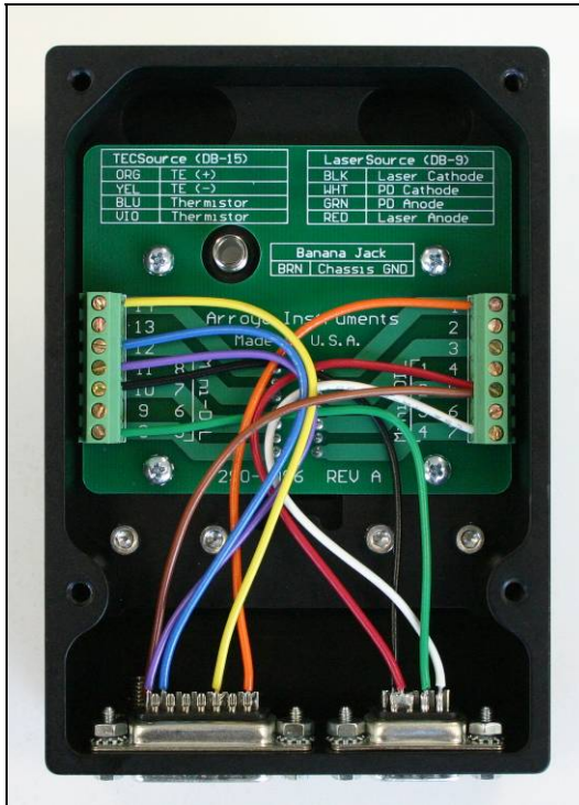
Internal Wiring Example
