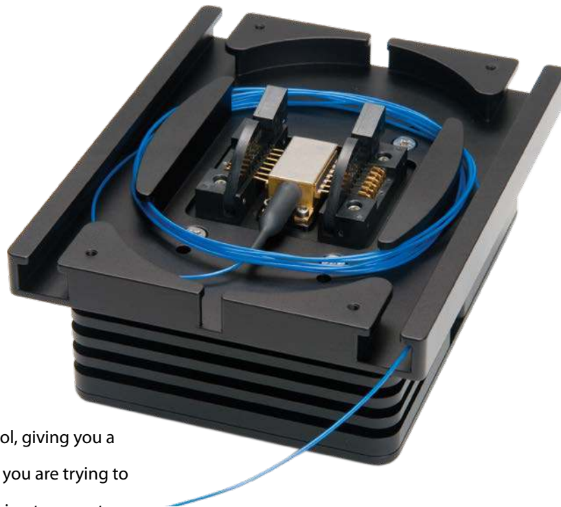
224 with opto-mech plate (cage system not included)
